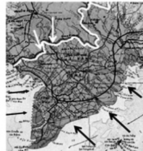
Fig.4. Three interference zones between fluvial and tidal processes
